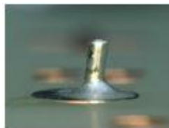
Dissatisfactory Insufficient solder
