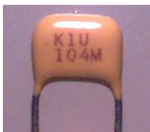
Kemet Ceramic Coated Radial Capacitor 0.1uF
