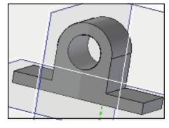
Modeling the bearing is done by selecting the inner circles. The bronze bearing is created as a separate part.
