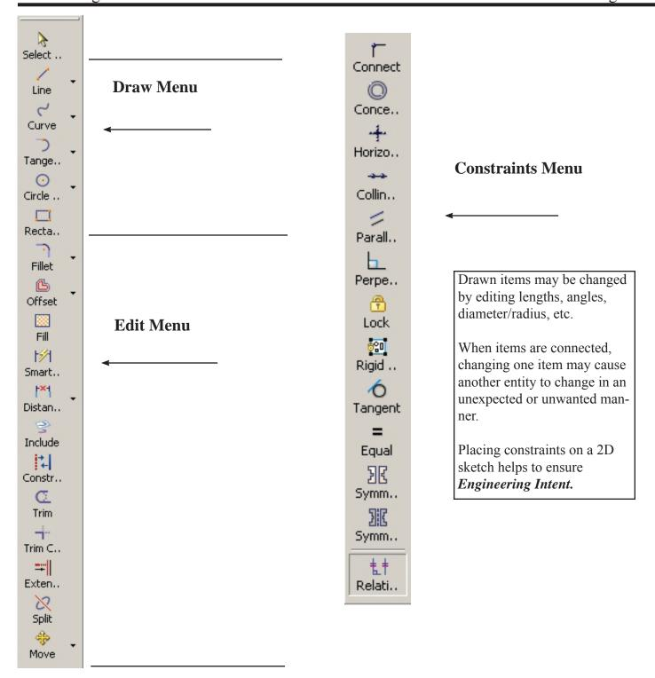
Constraining sketches is an important step in the design process. Many features may be changed as the design evolves. Making sure the master sketch changes in a predictable manner is critical.
